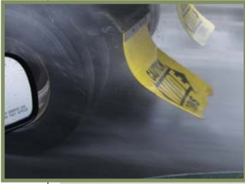
Air passes through the Eco-flaps, top, saving fuel and cutting splash and spray compared to the traditional mudflaps in the bottom photo.
